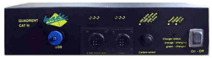
The standard measurement program configured at the factory is detailed below—This can be easily modified by the user Star connection, Nominal Voltage 230 Vrms, Nominal current 5Arms, Integration period 10 minutes, Network Frequency 50 Hz. Voltage transformer 230/230, voltage hysterisis 10%, current hysterisis 10%. The power quality thresholds are those of EN50160, and the bargraphs are 200 to 250 Vrms, power factor 0.5 to 1, frequency 49.5 to 50.5. Harmonics 2 to 24.
