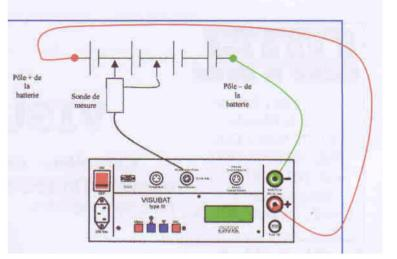
**Measurement Principle**—The impedance is measured by the capacitive coupling of an alternating current source to the battery, followed by measurement of the alternating voltage across the probes.
