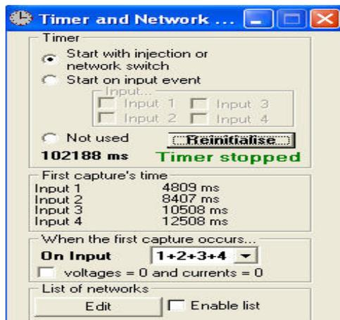
Switching from a healthy state to an out-of-limits state (left), displays the response time of the protection device on the screen (below)
