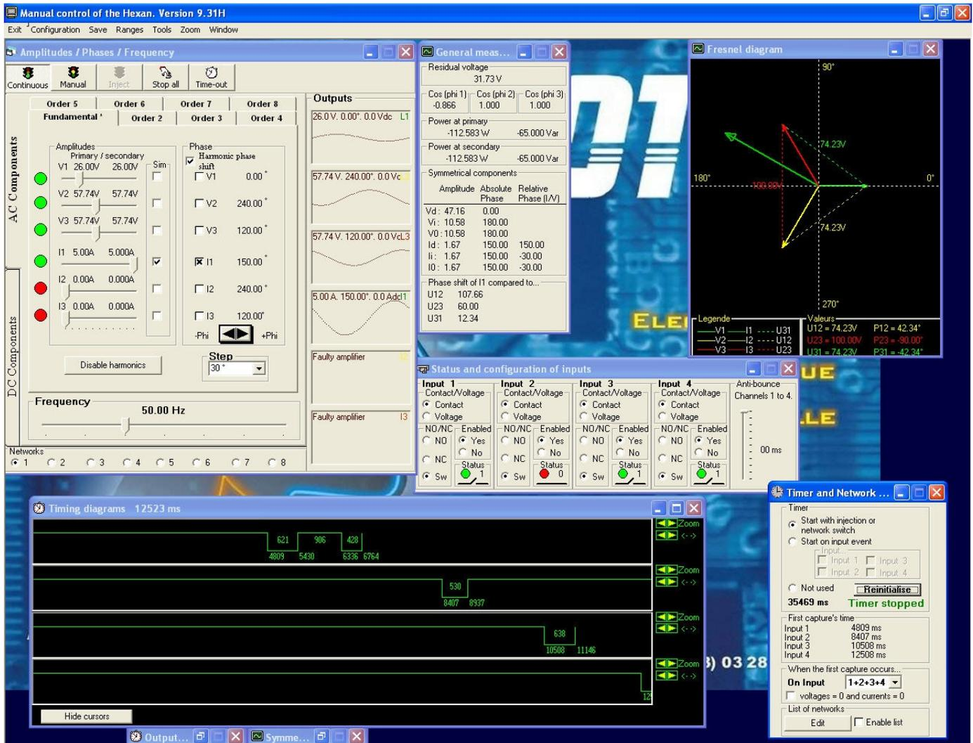
The **MANUSOFT** software package is supplied free with every **HEXAN** and **POWHEX** and there is no limit to the number of computers into which it can be loaded. As it is extremely easy to use, no computer expertise is required to benefit from all the test set's features and to fully test all commonly encountered relay types, and then produce professional test reports.
