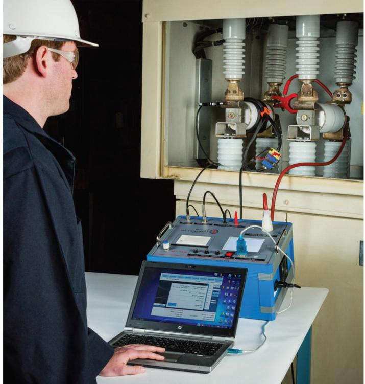
It is well known that the vacuum interrupter chambers work well until they no longer work, sometimes with disastrous results. The MAC TS4 offers a means of predicting the remaining life of vacuum bottles, without the need for dismantling for laboratory testing.
