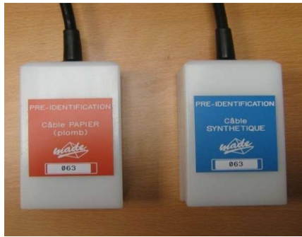
Sensor for «Identification in short-circuit ».
