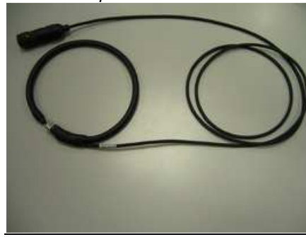
Sensor for «Core identification, short-circuited ends »
