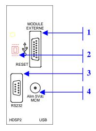
Sub D 15-pin connector for connection to the external module. This connector contains the amplifier control signals at a low level (7.07Veff) and the control signals for the external modules.
