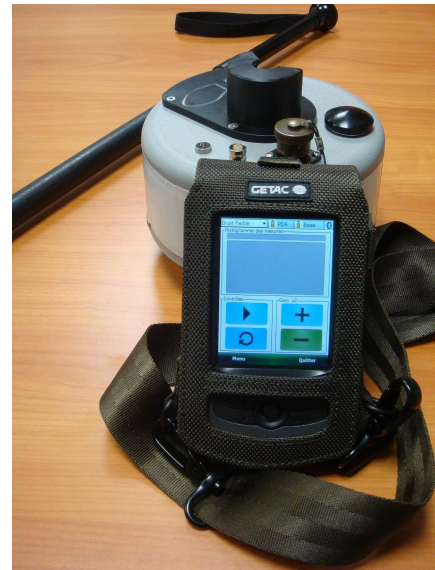
ABOVE - the receiver set with colour touch-screen and the robust detector foot with its removable handle RIGHT - The handheld communicates easily with the detector foot by Bluetooth.
