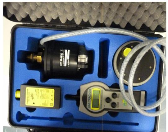
The system works best on a tarmac road or pavement, but we now have techniques to enable it to locate pipes under unmade ground. It can also be used for the identification of a metal pipe among others by placing the detector directly on the metal pipe.
